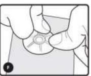
**Step F:** Press down on the snap to secure to substrate. Work all the way around the snap and in the center.
