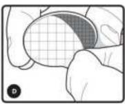
**Step D:** Remove liner from the back of disk.
