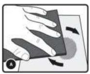
**Step A:** Some surfaces may need to be abraded using a mild abrasive pad prior to cleaning
