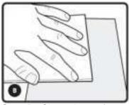
**Step B:** Clean the surface using either a solvent or alcohol wipe.
